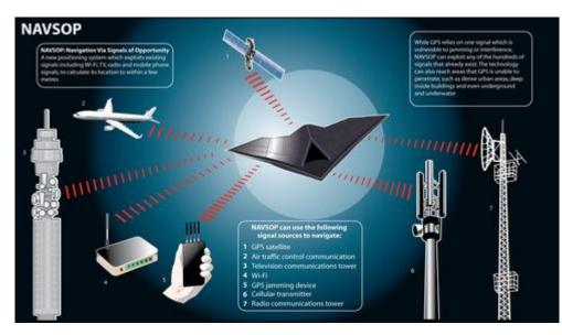
BAE Systems UK has unveiled its latest research on an advanced positioning system that exploits existing transmissions such as Wi-Fi, TV, radio and mobile phone signals, to calculate the user's location to within a few metres.
