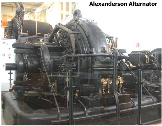
machine was invented in 1904 by Ernst Alexanderson to generate HF alternating current up to 100 kHz, for use as a radio transmitter. It was one of the first devices capable of generating the continuous radio waves needed for transmission of AM (sound) by radio, and was used for a short period through the 1920s in the first AM radio transmitters, until it was replaced by vacuum tube transmitters.
